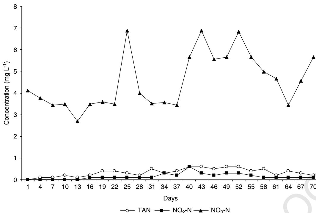
**Figure 2.** TAN, NO<sub>2</sub>-N and NO<sub>3</sub>-N concentrations in the rearing water of *P. monodon* maturation system integrated with packed bed bioreactor during 70 days operation.
