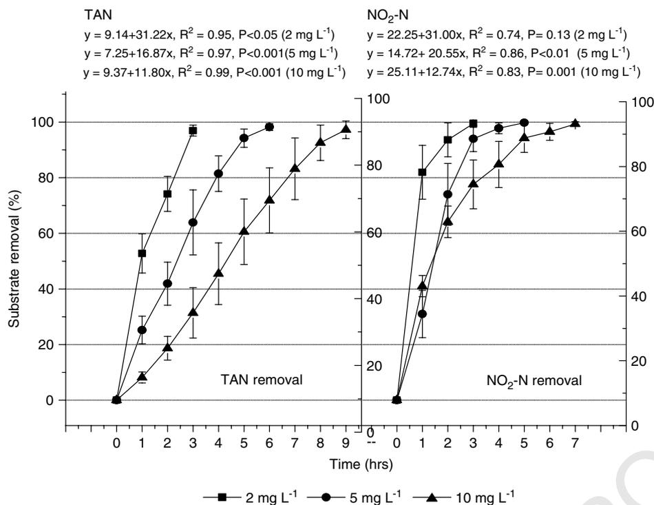
Figure 5. Percentage TAN and NO<sub>2</sub>-N removal rates in the reactor system at initial substrate concentrations of 2, 5 and 10 mg L<sup>-1</sup>.
