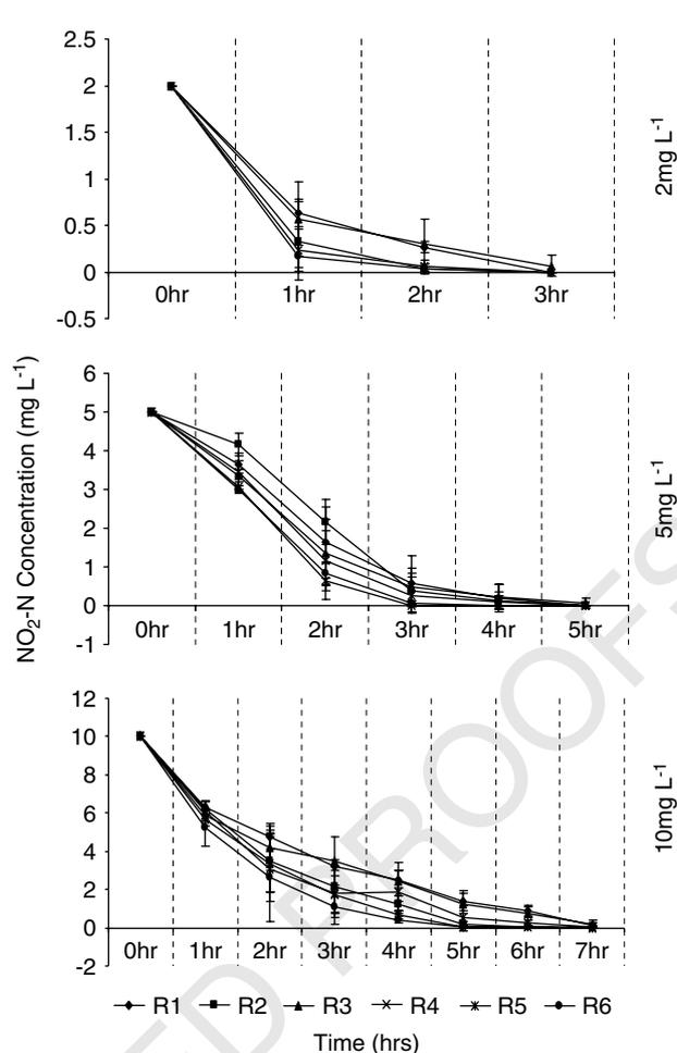
**Figure 4.** NO<sub>2</sub>-N consumption in the reactors fed with NO<sub>2</sub>-N concentrations of 2, 5 and 10 mg L<sup>-1</sup>.
