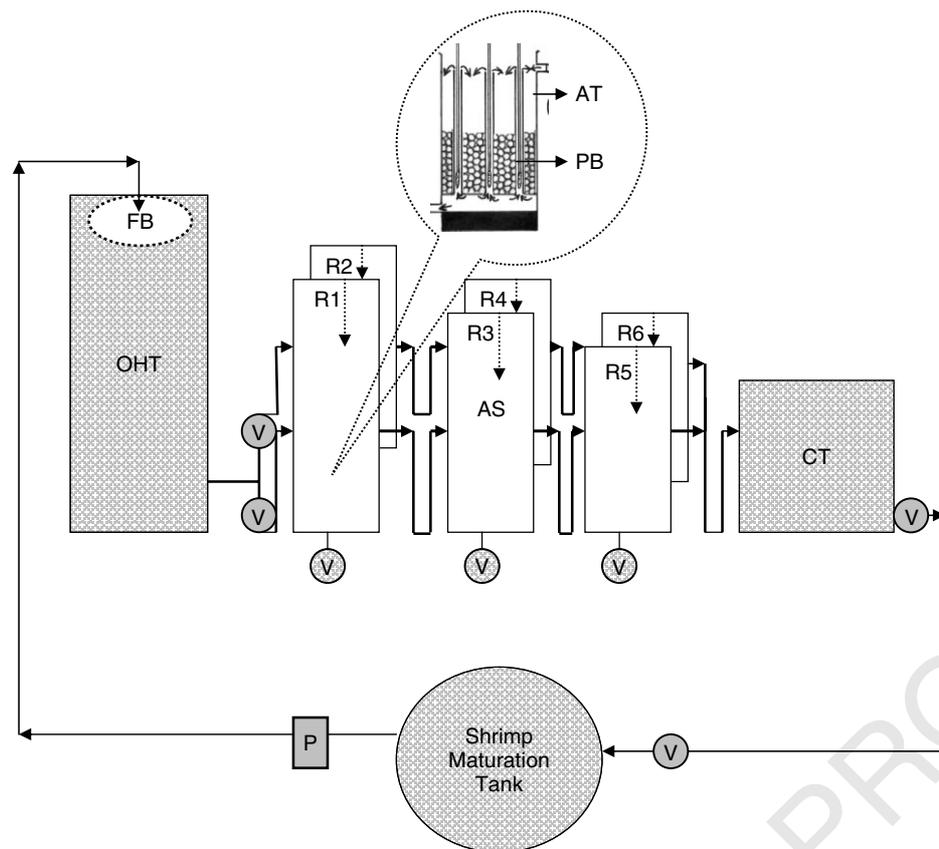
**Figure 1.** Packed bed bioreactor connected to a shrimp maturation system. AS–aeration supply; AT–aeration tube; CT–collecting tank; FB–filter bags; OHT–Overhead tank; PB–polystyrene beads; P–pump; R1–R6 – reactor R1–R6; V–valves.
